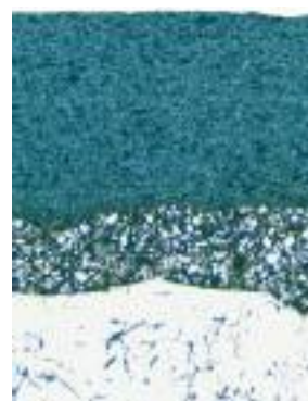
Cross section of Flygt epoxy coating
