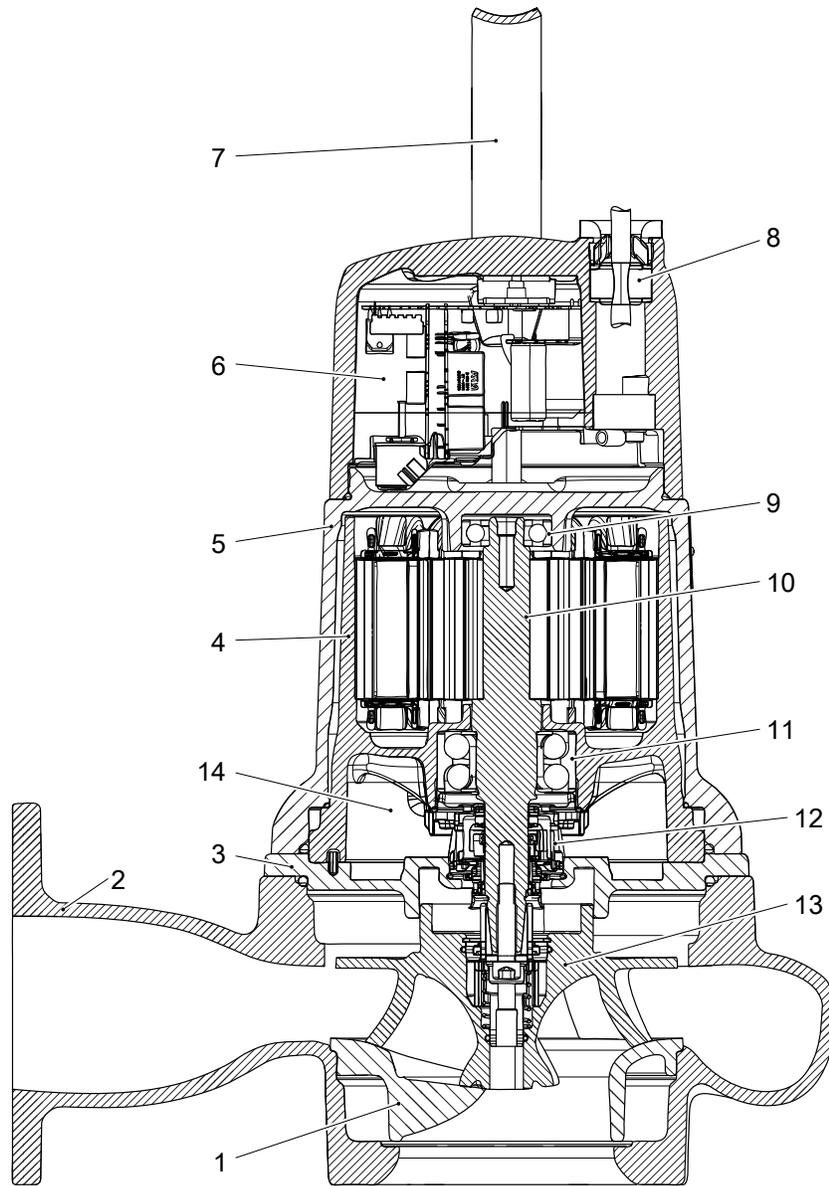
Figure 1: Outer casing of drive unit: Gray iron
