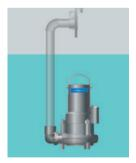
Stationary wet installation suspended from the discharge pipe. The quick connection joint has an integrated non-return valve applicable for Flygt Compit pump stations.
