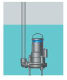
**F-installation**Free standing, the pump is equipped with supporting legs. Can be connected to hose or pipe.
