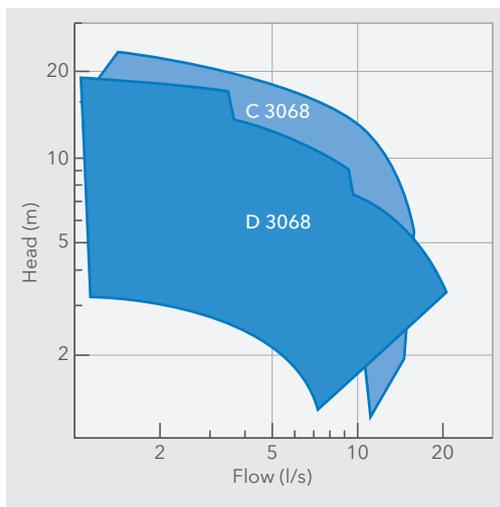
C = Kanalradpumpen D = Freistromradpumpen
