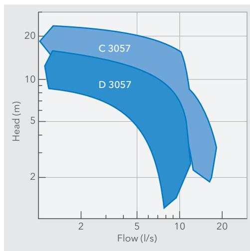
C = Kanalradpumpen D = Freistromradpumpen
