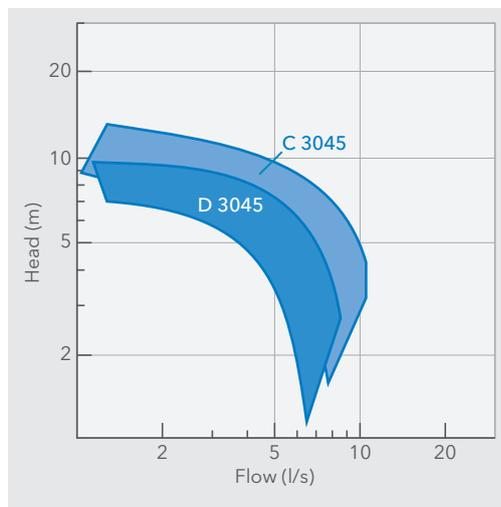
C = Kanalradpumpen D = Freistromradpumpen
