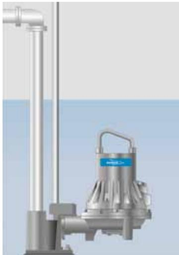
Stationary wet installation with guide bars and automatic discharge connection bolted to the sump floor. When lowering a pump with guide bars, the pump automatically locks to, and is released from, the discharge connection.
