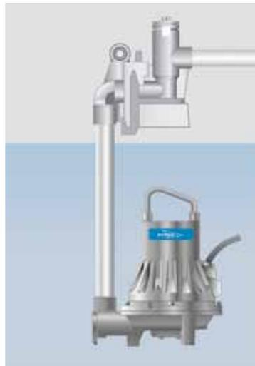
Stationary wet installation with the pump suspended from the discharge pipe. The quick connection joint has an integrated non-return valve.
