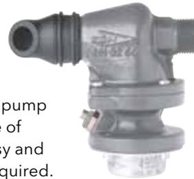
The flush valve provides a powerful cleansing jet stream to clean the wet well at the start of each pumping cycle. This reduces the risk of solids build-up and increases both pump efficiency and service life.
