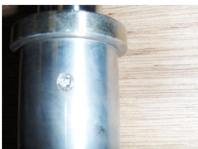
Afgebroken machine tap in asbus.
