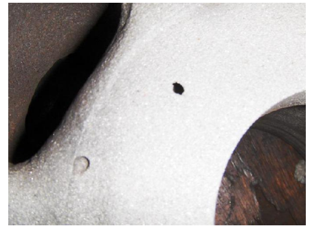
Gaten in pomphuis
