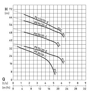
H = Total Head; Q = Discharge Volume. Curves to ISO 9906 (60 Hz available on request) N.B. please use the ABSEL program to validate pump selection.
